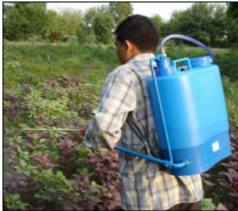
A backpack sprayer is a great tool for applying herbicide to unwanted plants in the prairie.
